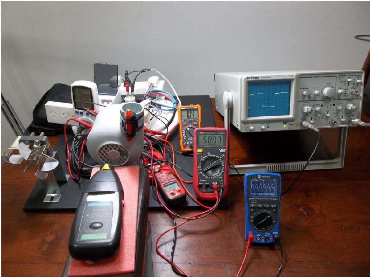
Figure nº 15. Test bench connected to SARS-CoV-2 or Covid-19 (Coronavirus) stale air extractor/centrifugal blower motor: Turbo. With digital multimeter (volt meter in AC), clamp meter (current intensity meter in AC), frequency meter (Hertz meter), laser photometer (speed meter in RPM), digital oscilloscope waveform meter the alternating current in voltage ( V_{peak-peak} , V_{avg} , V_{rms} ), to calculate the harmonic distortion crest factor, analog oscilloscope for qualitative observation of the THD (harmonic distortion of the alternating current), wattmeter (active power meter in watts or watts), power factor (cosine \phi ), power-meter (active energy consumption meter in kilowatt-hours: kwh). Source: Own elaboration.
