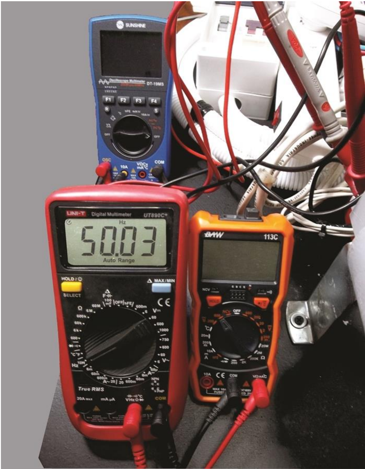
Figure nº 16. View of the frequency meter turned on indicating the 50 (Hertz) of the alternating current (AC), next to the digital multimeter (voltmeter) turned off. Source: Own elaboration.
