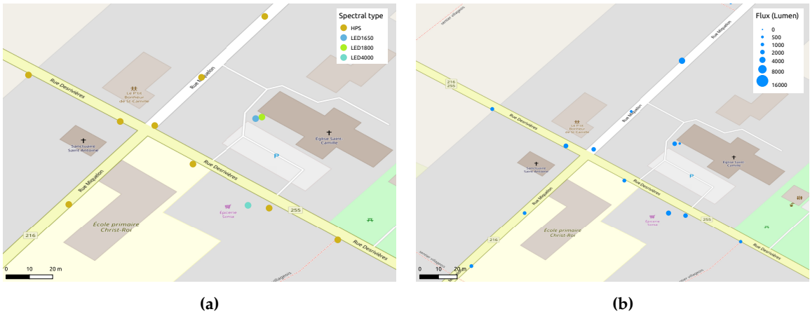
Figure 6. Detected spectral types and luminous fluxes in central part of Saint-Camille, Québec, Canada.
