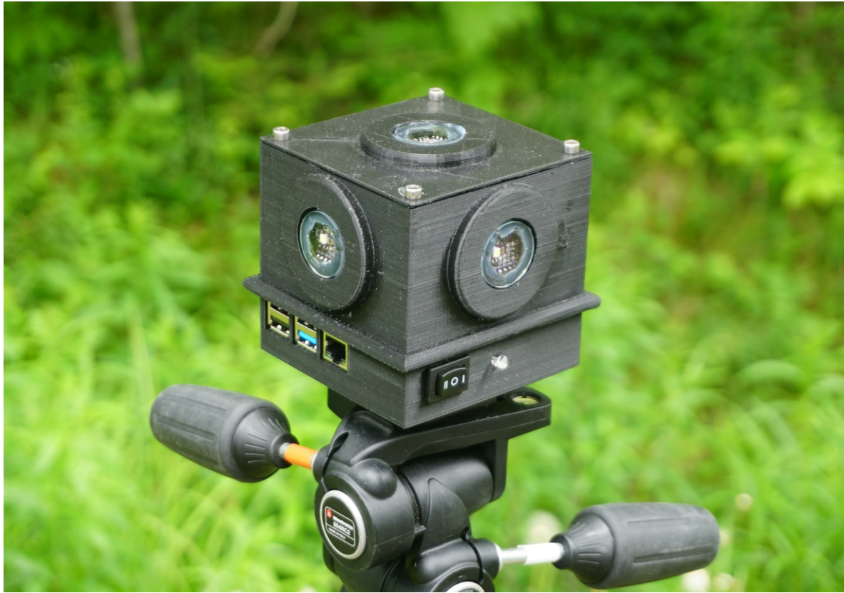
Figure 1. The LANcube v2 radiometer. On the bottom of the left face, are the USB and ethernet ports and on the right face one can see the operating switch and status RGB LED. At the center of each face lies a light color sensor. The size of the LANcube v2 is 9x9x9 cm.
