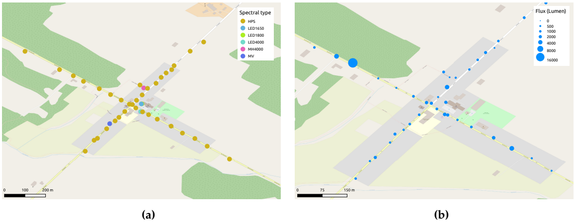
Figure 5. Detected spectral types and luminous fluxes in Saint-Camille, Québec, Canada.
