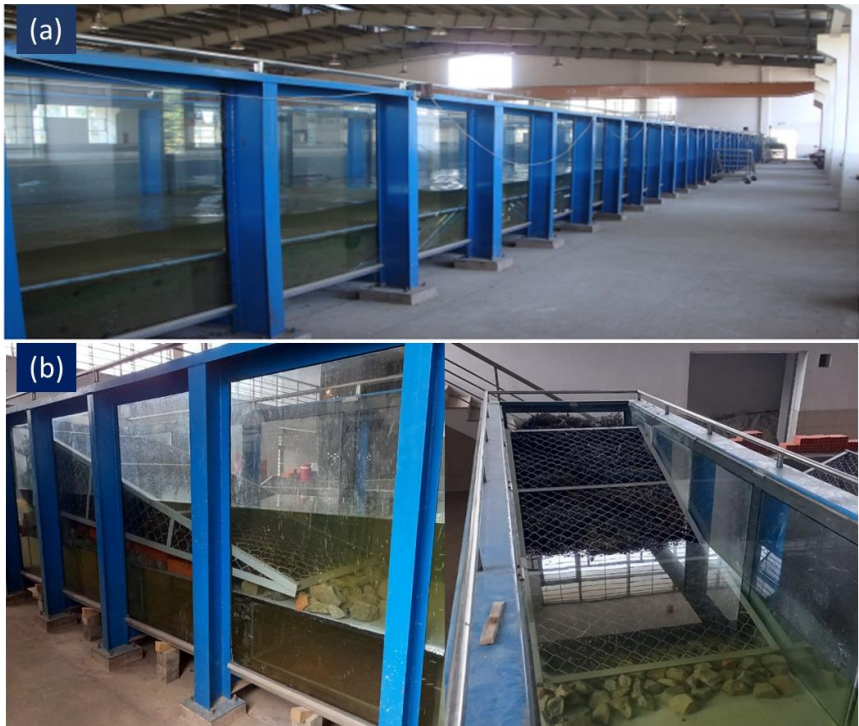
Figure 2. The wave flume house (a) and absorber at the lee side of wave flume (b).
