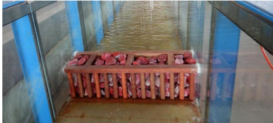
Figure 5. Experimental pile-rock breakwater set up in the wave flume at Laboratory.
