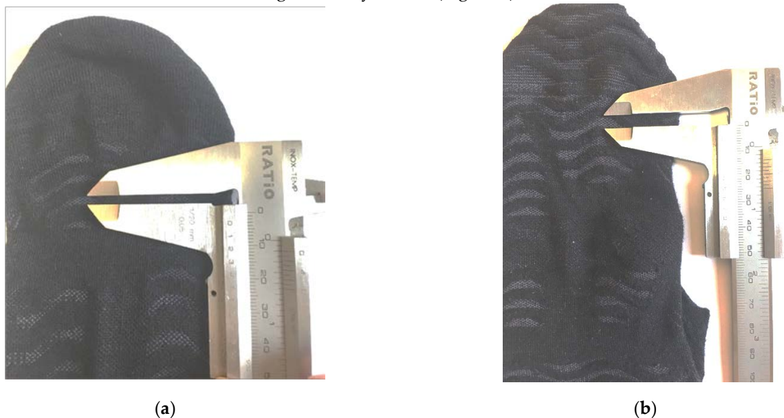
Figure 1. Configuration of plantar ribbing in sock models AWC 1 (a) and AWC 2.1 (b).
