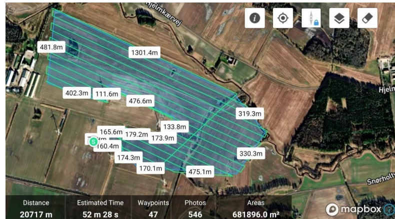
Figure 1. Example flight route mapped in DJI Pilot App [42]. The blue area indicates the ground area covered on the aerial images and the green lines show the flight route with distances between mapping points annotated along the route.
