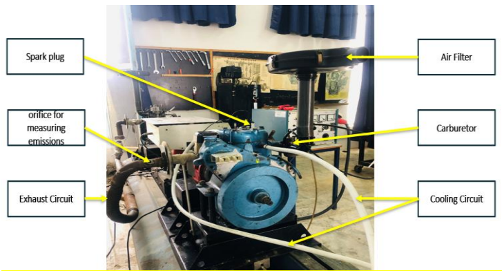
Figure 2. Single-cylinder SI engine on a test bed.
