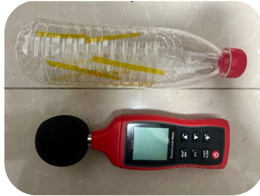
Figure 4. Handmade microphone (up) and Sound level meter SLM (down).
