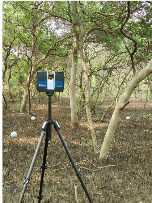
Figure 2. Laser scanning using FARO Focus S 350 Terrestrial Laser Scanner.
