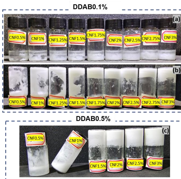
Figure SI1. CNF emulsion pictures of (a) the mixture of oil-water before homogenization, (b) CNFX%-DDAB0.1% and (c) CNFX%-DDAB0.5%.
