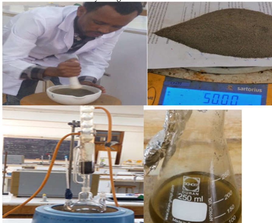
Figure 2. Size Reduction and balancing of the sample and Extracted oil from filter mud by using the Soxy let extraction method.
