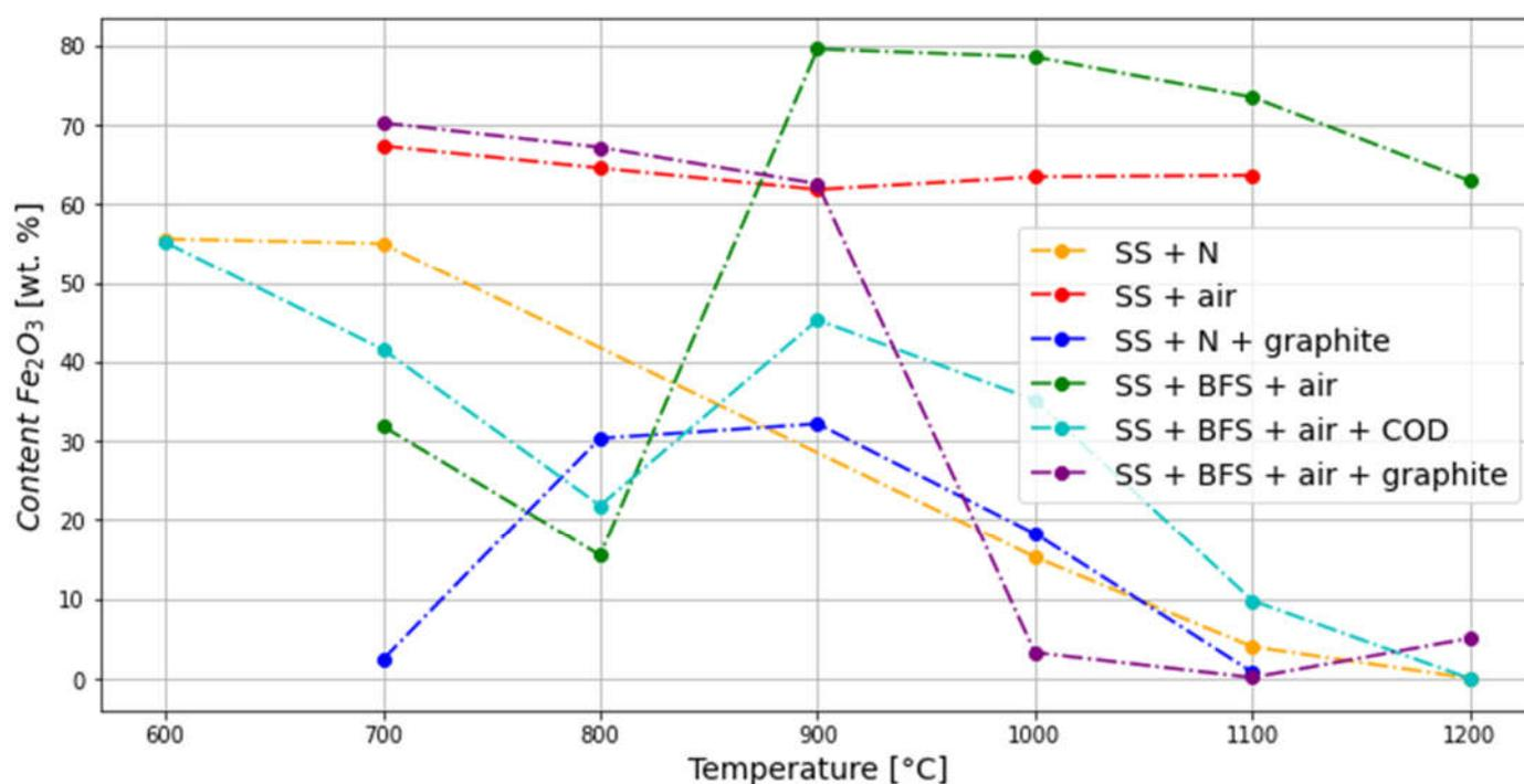
Figure 3. Effect of temperature, atmosphere and reducing element on Fe<sub>2</sub>O<sub>3</sub> content in sludge.
