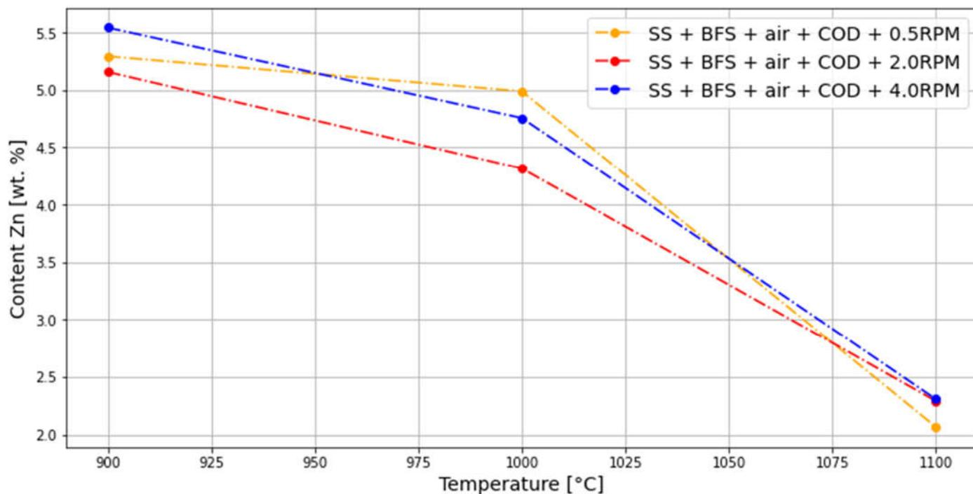
**Figure 8.** Effect of temperature, atmosphere and reducing element on Zn content in sludge in a mixture of steelmaking and blast furnace sludge in an atmosphere of air with coke oven dust, depending on the speed of rotation.
