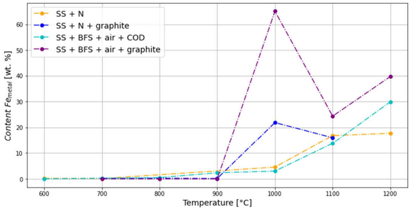
Figure 5. Effect of temperature, atmosphere and reducing element on metallic Fe content in sludge
