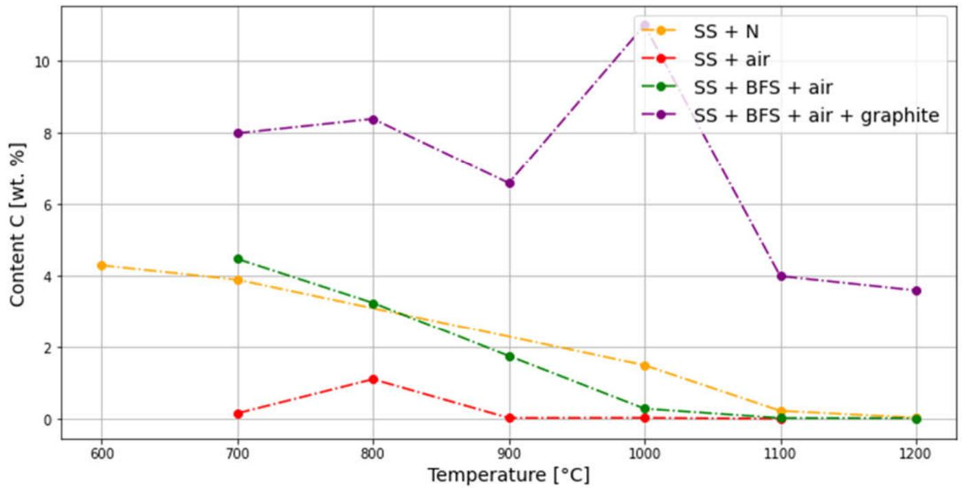
Figure 6. Effect of temperature, atmosphere and reducing element on C content in sludge
