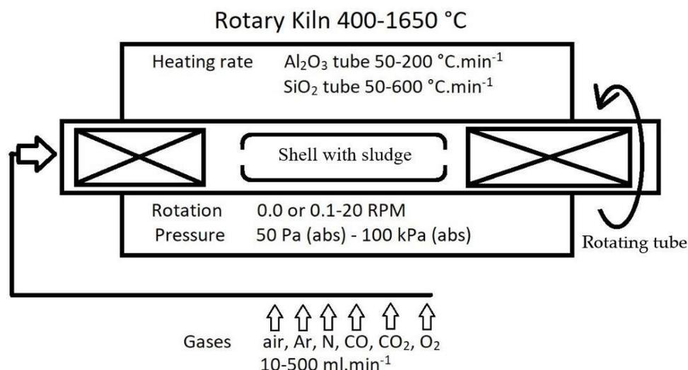
**Figure 2.** Experimental scheme of technological process in laboratory rotary kiln.
