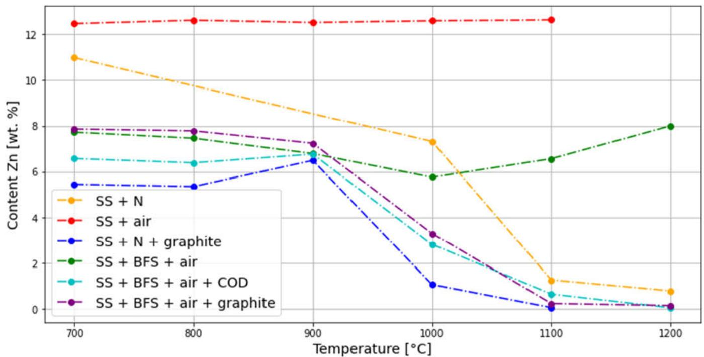
Figure 7. Effect of temperature, atmosphere and reducing element on Zn content in sludge
