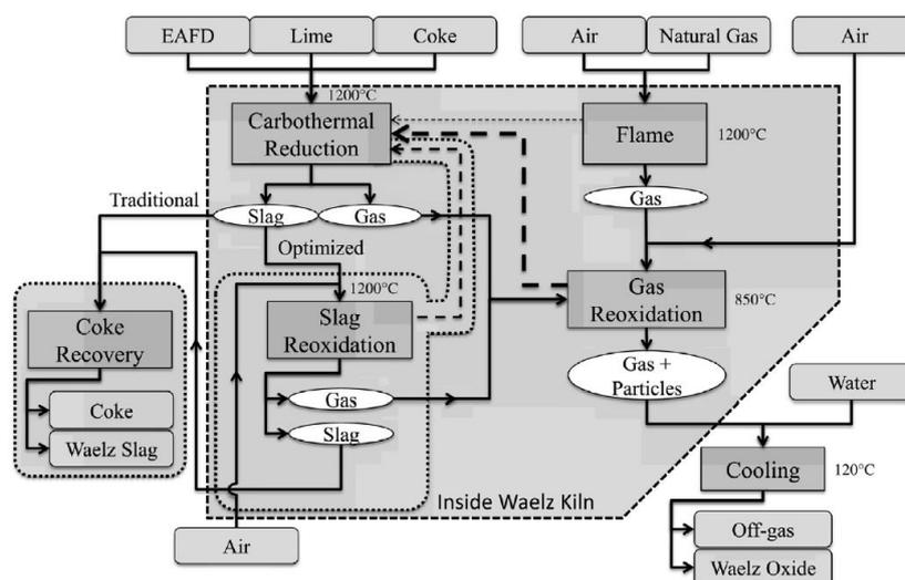
Figure 1. Schema of Waelz process [16]
