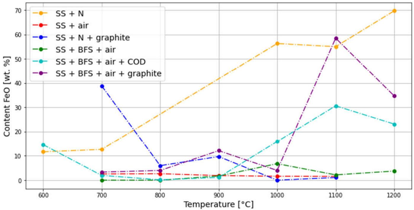
Figure 4. Effect of temperature, atmosphere and reducing element on FeO content in sludge.
