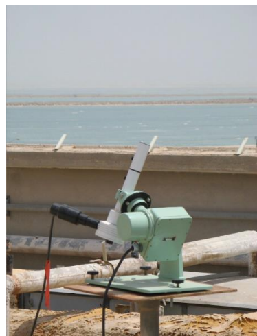
Figure 6. The normal incidence UVB measured by means of a Model 501A UV-Biometer mounted on an Eppley Solar Tracker Model St-1.
