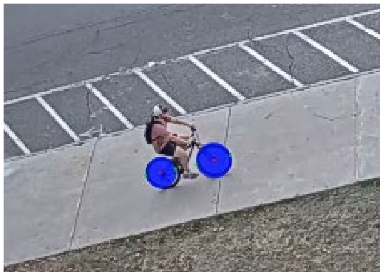
FIGURE 8 Detection of bicycle wheels using Hough transform
