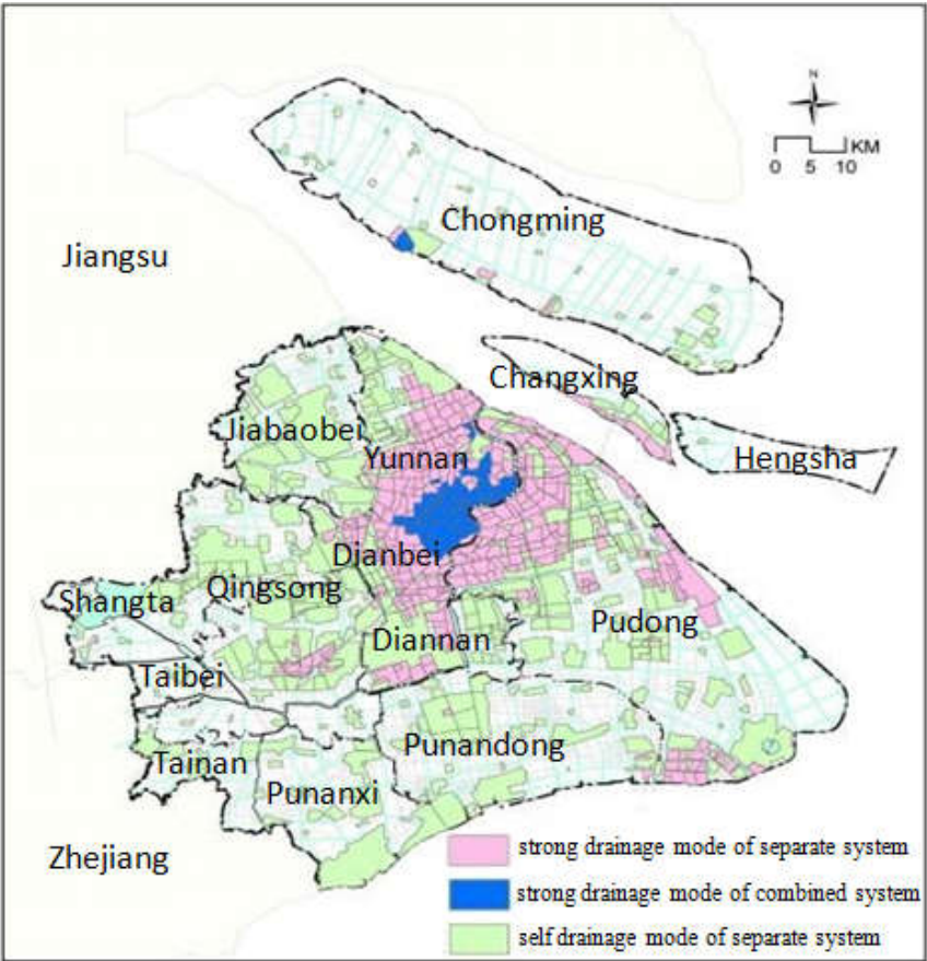
Figure 3. Drainage area zoning and their drainage mode in Shanghai.
