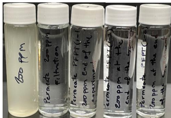
Figure A12: From left to right, feed 200ppm, no PFPT permeate, PFPT (1-1) permeate, PFPT (1-2) permeate, and PFPT (2-2) permeate
