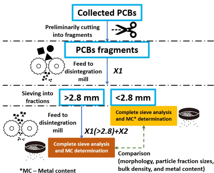
**Figure 3.** An applied disintegration-milling, sieving, and testing scheme show an approach for selecting fractions of powders from PCBs for metal content determination after one-step (X1) and double-step (X1(>2.8)+X2) disintegration-milling.
