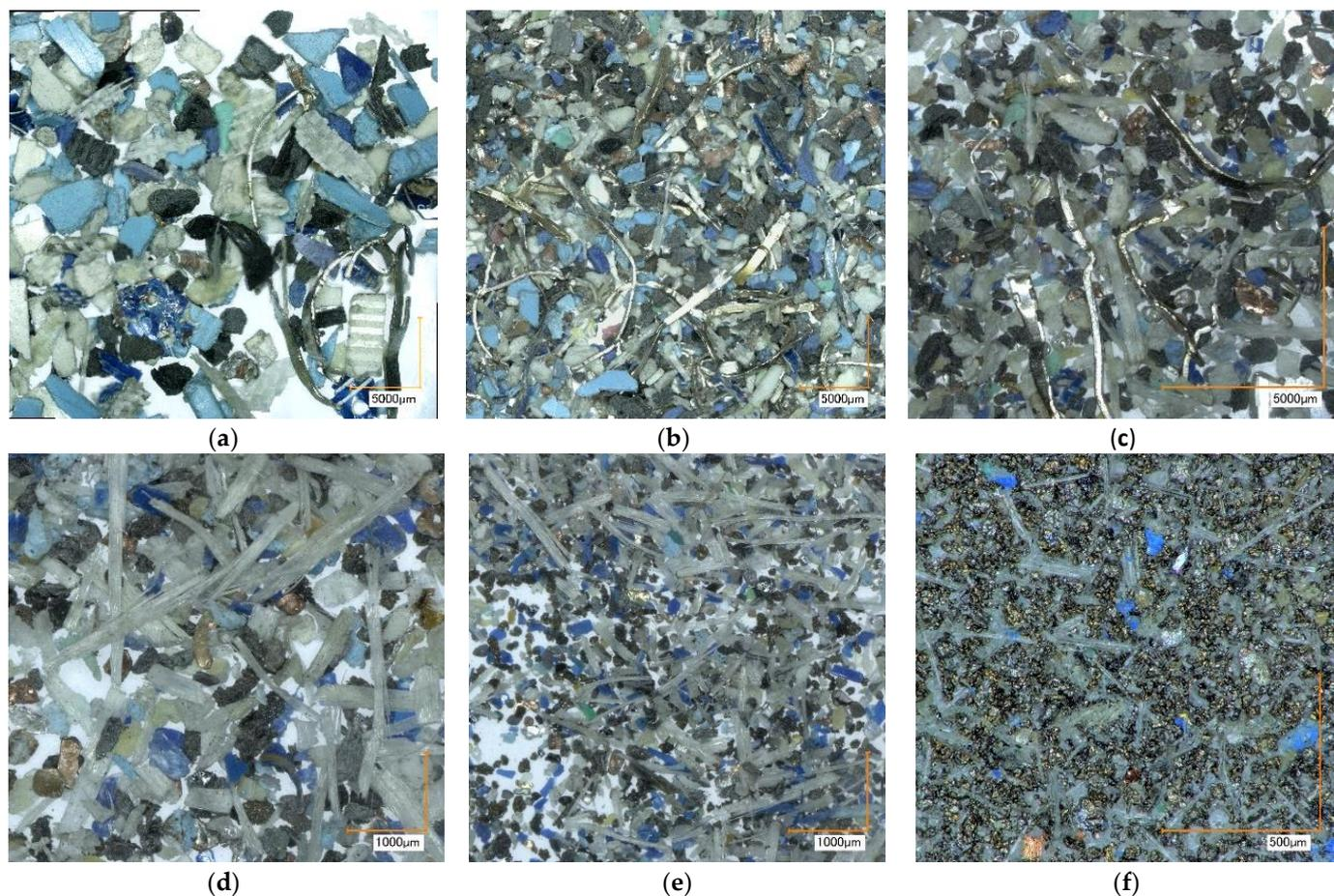
**Figure 5.** Optical images of the fractions 1.4–2.8 mm (a), 0.711–1.4 mm (b), 0.355–0.711 mm (c), 0.355–0.18 mm (d), 0.09–0.18 mm (e) and <0.09 mm with significantly lower fiberglass concentration (f) after one-step milling (X1).
