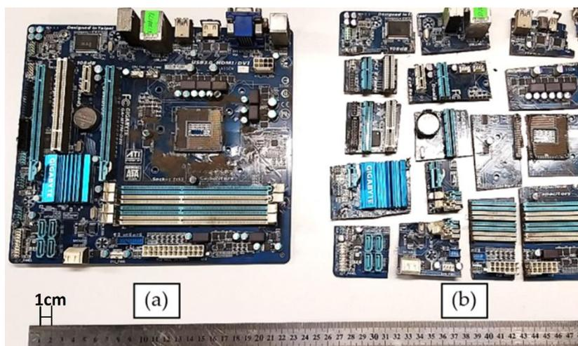
**Figure 1.** As-received computer motherboard (a) and after cut into pieces before milling (b).
