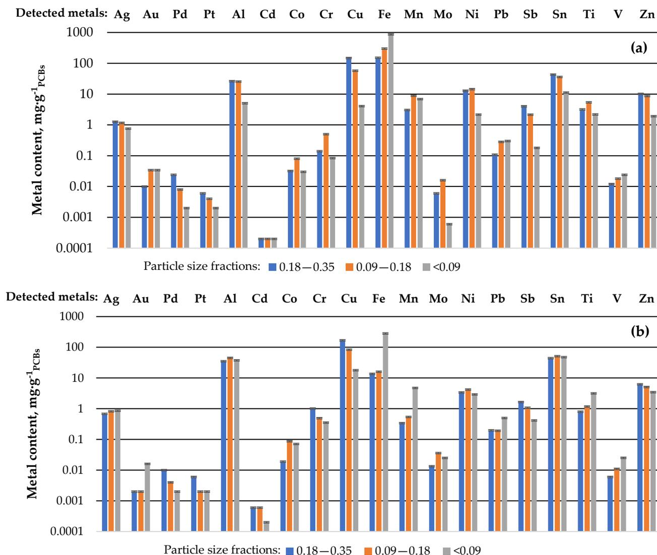
**Figure 4.** Dependence of element composition of milled fraction by particle size distribution for X1 (one-step) (a) and X1(>2.8)+X2 (double-step for >2.5 mm fractions from first milling) (b) millings.
