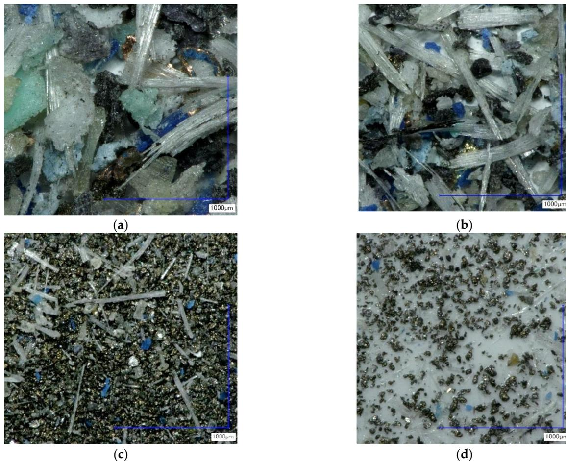
**Figure 6.** Optical images of the fractions 0.711–1.4 mm (a); 0.355–0.711 mm (b); 0.09–0.18 mm (c); and <0.09 mm (d) after double-step milling ( $X1(>2.8)+X2$ ) of fraction >2.8 mm collected from the one-step milling.
