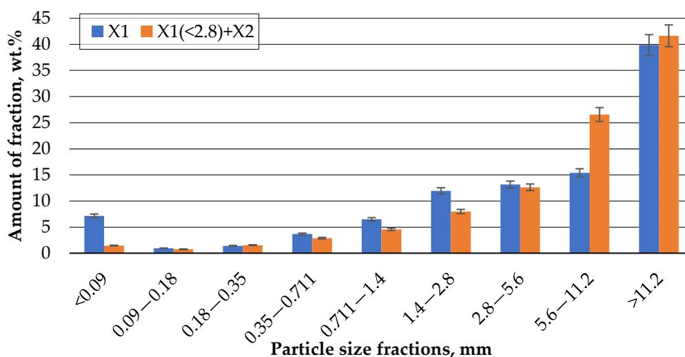
**Figure 7.** Particle size distribution of the disintegration-milled PCBs after first “ $X1$ ” and second milling of the fraction with particle sizes larger than 2.8 mm from first milling designated as “ $X1(>2.8)+X2$ ”.
