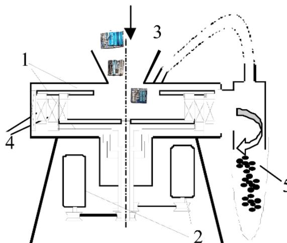
**Figure 2.** Schematic representation of preliminary size reduction centrifugal-type mill DSL-350. Equipment: 1—rotors; 2—electric drives; 3—material (PCBs) supply; 4—horizontally oriented grinding elements; 5—output.
