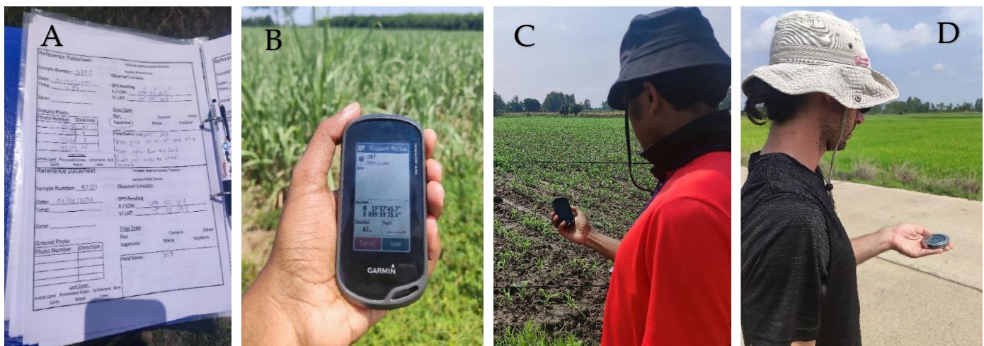
Figure 5. Manual data collection using GPS: A. Reference data sheet; B. Handheld GPS device; C. Using mapping grade GPS device; and D. Finding the North direction.
