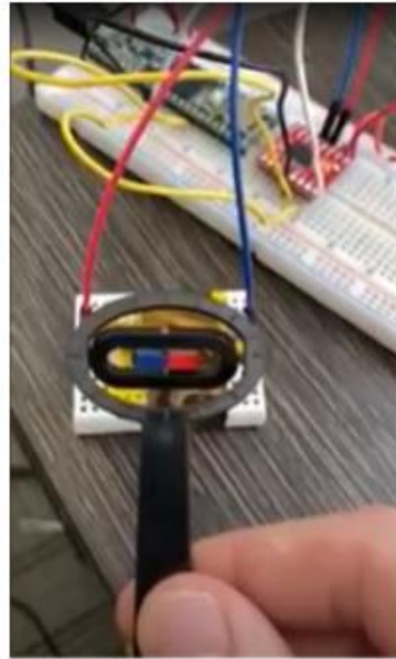
Figure 34: The gyrocompass measuring the magnetic field of the torque coil
