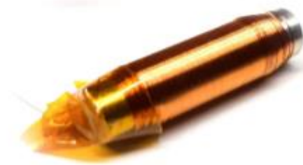
Image 4: Torque coils made in house
