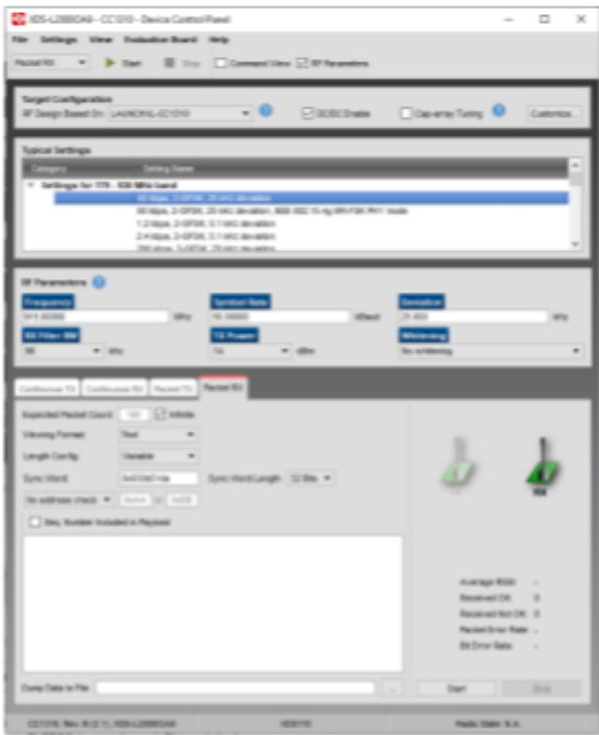
Figure 8: Configuring the PacketRX in SmartRF Studio 7
