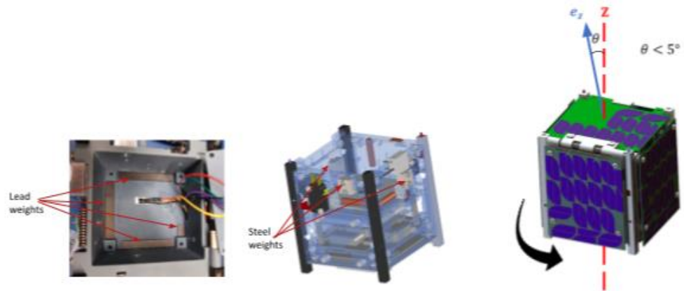
Figure 27: Passive ACS techniques used in Alpha Photo credit Josh Umaksky-Castro
