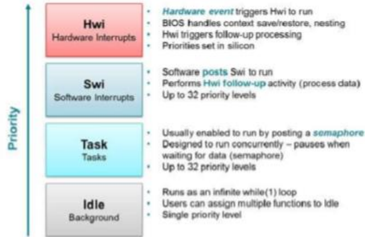
Figure 9: TI-RTOS Kernel priority levels. Image credit from TI (link in references)
