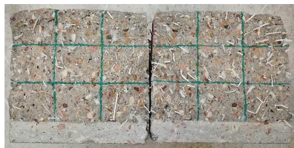
Figure 3. Analysis of the fracture section of specimen 7PF-1 (Shotcrete sample).
