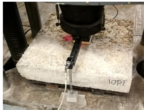
Figure 4. 10PF plate test assembled according to EN 14488-5 [22].
