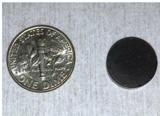
Figure 2. The fabricated sintered CAO pellet.
