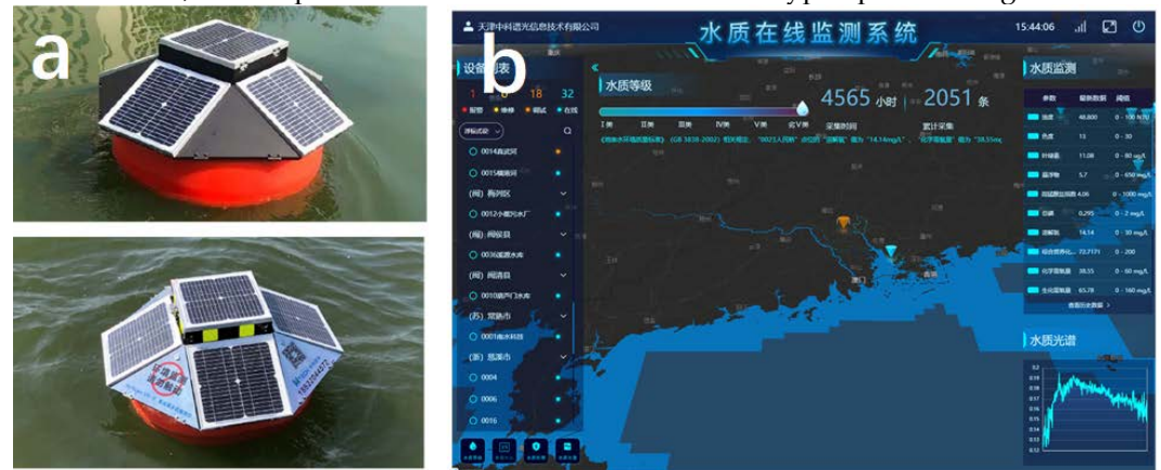
Figure 3. The system is composed of intelligent water quality spectrometer and data analysis cloud service platform. (a) The water quality spectrometer is fixed on the water surface, collects spectral data regularly, and transmits it to the cloud service in real time through 4G / 5G network. (b) The system supports cloud data storage, statistical analysis, and supports real-time viewing on the user's client.
