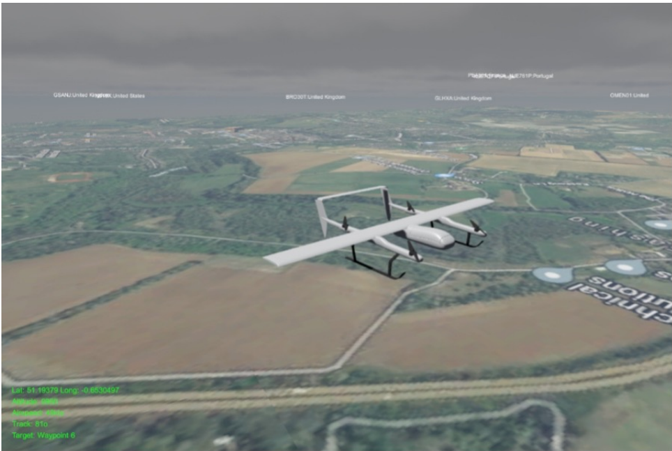
Figure 8. FUSE simulator showing Muglin UAS flying over Google Earth terrain with ADS-B Information in White
