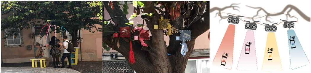
Figure 8. Public installation using four proximity sensors placed inside foliage with hanging ribbon. Sensors are physically separated by sensing trajectories, identified by colour.
