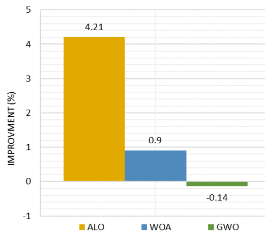
Figure 11. Comparison of ALO, GWO, and WOA for input reduction on SSTs
