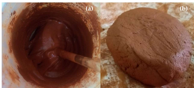
Figure 4. Processing of pre-treated Red Mud fine powders with 1.0 M HCl solution [Red Mud fine powders mixed with 1.0 M HCl solution (a); Red Mud pasty cake (b)].
