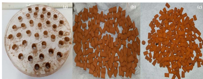
Figure 5. Production of activated Red Mud Material pellets before and after calcination [Acrylic mold (a); Red Mud pellets before calcination (b); Red Mud pellets after calcination (c)].
