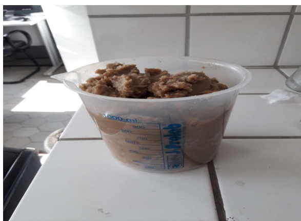
Figure 2. Pre-treated residual fat used as feed material by thermal catalytic cracking at 450 °C, 1.0 atm, 0.0, 5.0, 7.5, and 10.0% (wt.) Red Mud pellets activated with 1.0 M HCl, using a catalyst fixed bed reactor, in semi pilot scale.
