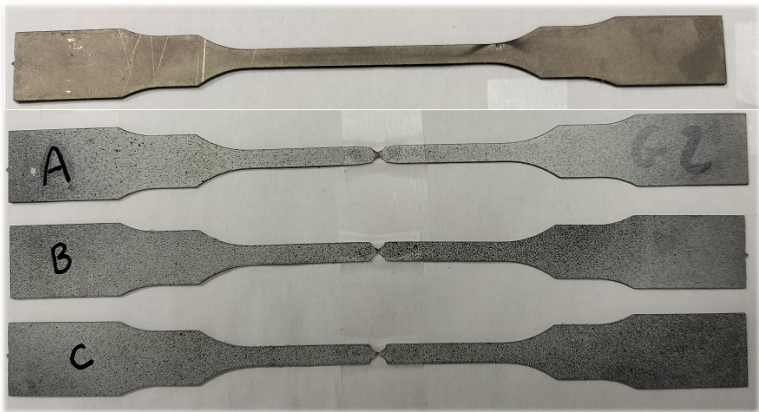
Figure 6. Notched and different unnotched specimens used in tensile tests
