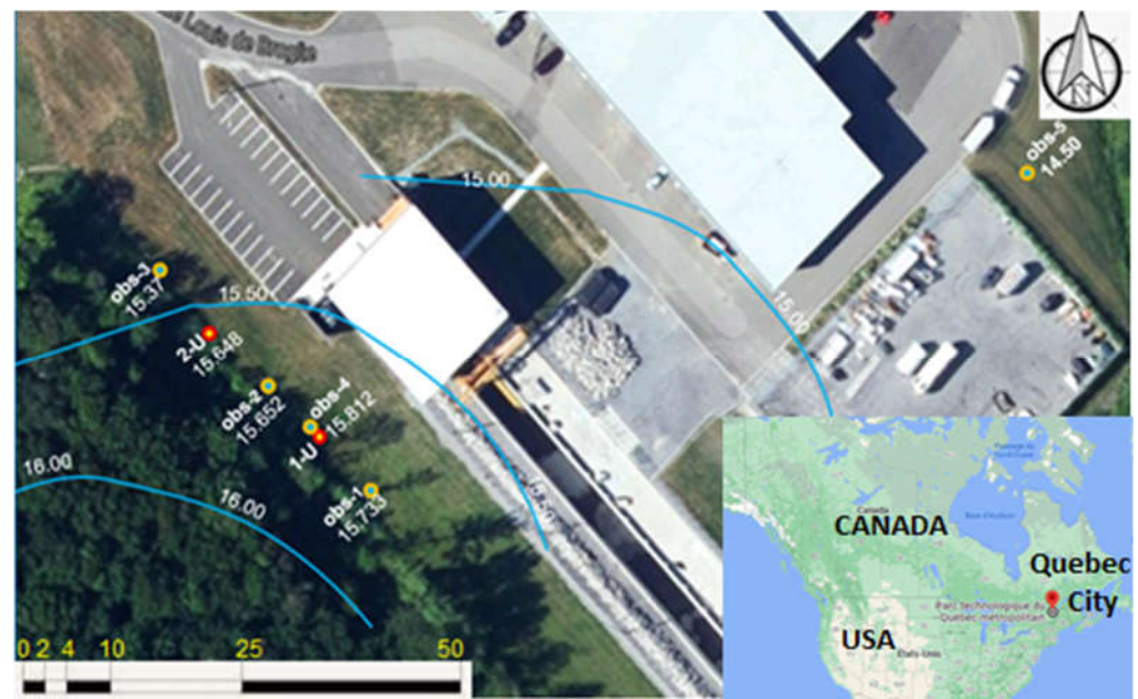
Figure 4. Geothermal experimental site at INRS (Quebec City). Numbers beside boreholes (obs and U) in white and along blue lines indicate elevation of the water table in meter above the sea level and local potentiometric level, respectively [7]. Obs are for open observation wells, while 1-U and 2-U are the borehole heat exchangers.
