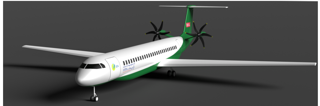
Figure 1. SE 2 A short range all-electric aircraft [2].
