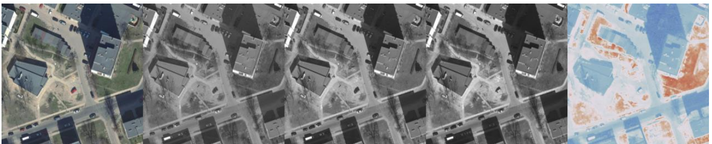
Figure 3. Visualization of a dataset item. From the left to right: RGB composition, R, G, B bands that form the input tensor and NDVI which serves as a target tensor. Source: own elaboration based on Geoportal [40].
