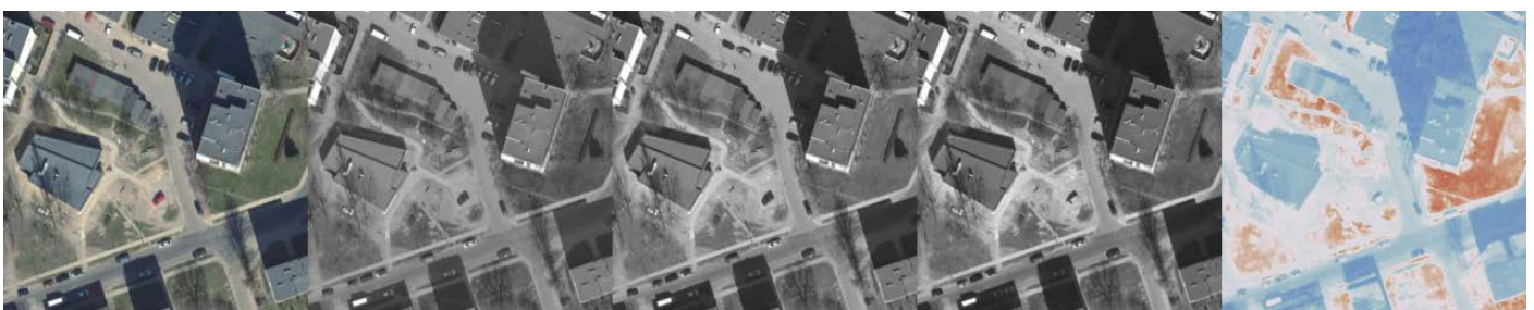
Figure 3. Visualization of a dataset item. From left to right: RGB composition, R, G, B bands that form the input tensor and NDVI, which serves as a target tensor. Source: own elaboration based on Geoportal [40].
