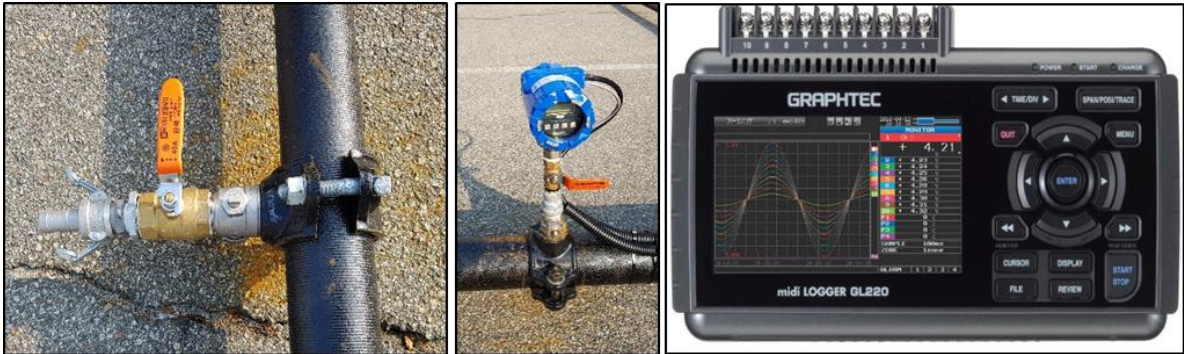
Figure 3. Valve for Leak and Transient Simulation, Pressure Transmitter, and Data Logger.
