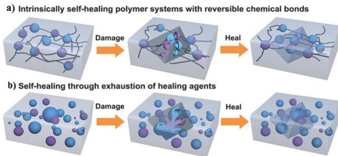
Figure 2. Intrinsically encapsulated self-healing systems Copyright Wiley, 2009 [7]
