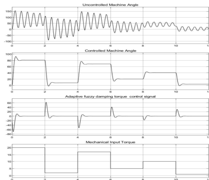
Figure 20. Fuzzy controller test for damping mechanical angle oscillation with mechanical torque input from 0 to 20.
