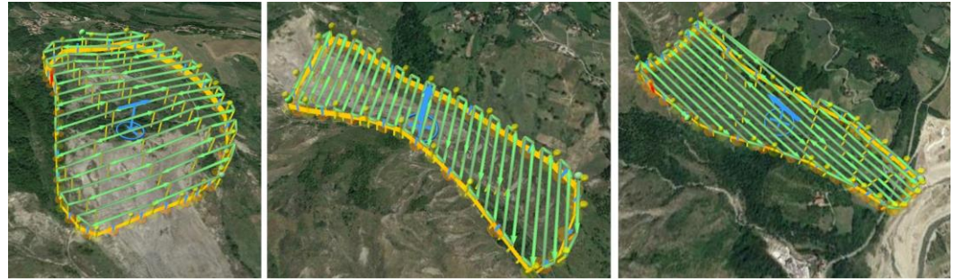
Figure 5. Flightplans of the landslide's top part (left), median part (centre), the bottom part (foot).
