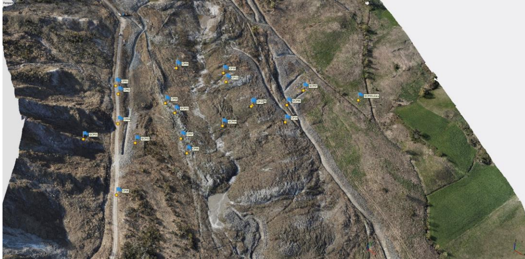
Figure 10. Dense point Cloud of the central part of the study area (Colata). The numbered flags on the ground surface represent the ground control points used for the bundle adjustment process.
