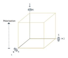
The piezoelectric effect is pronounced in different directions along the crystal. The reference axis, axis 3, is always taken along the axis of poling. Axis 1 and 2 in such a way that they form a coordinate system with axis 3. The shearing or twisting movement along the axes is referred to as 4, 5, 6 as shown in the figure.
