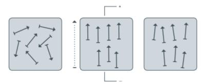
Piezoelectric material is made up of smaller electric dipoles which are in a random orientation resulting in a net-zero dipole moment. However, if an electric field is applied across the piezoelectric material the dipoles tend to align and result in a net dipole even after the removal of the electric field.
