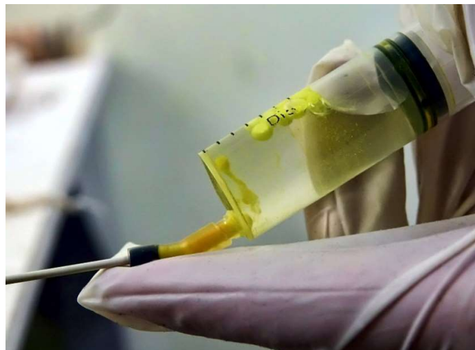
Figure 7. \text{H}_2\text{S} sampling into 1N \text{Cd}(\text{NO}_3)_2 solution using a plastic medical syringe through a ceramic capillary.
