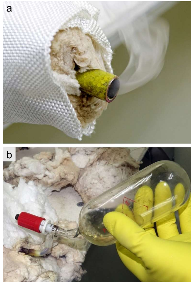
Figure 6. Sampling the total gas sampling using “Giggenbach bottle”. A – Gas escape from the cold end of the sublimate-collection tube; yellow deposits of sulfur are visible. B – Gas sampling via a ceramic capillary into 4N KOH solution.
