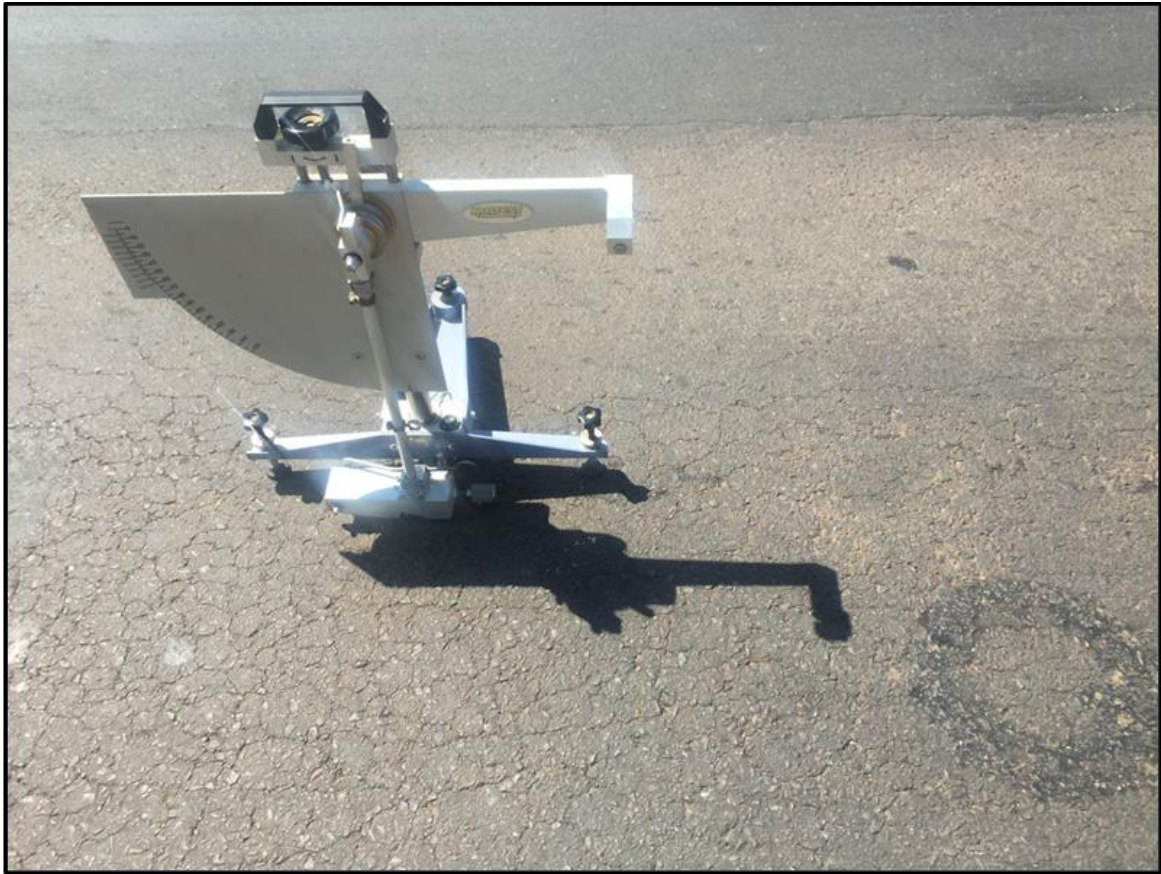
Figure 11: Skid resistance testing done before and after application of a clear-seal [18] (refer Acknowledgements).
