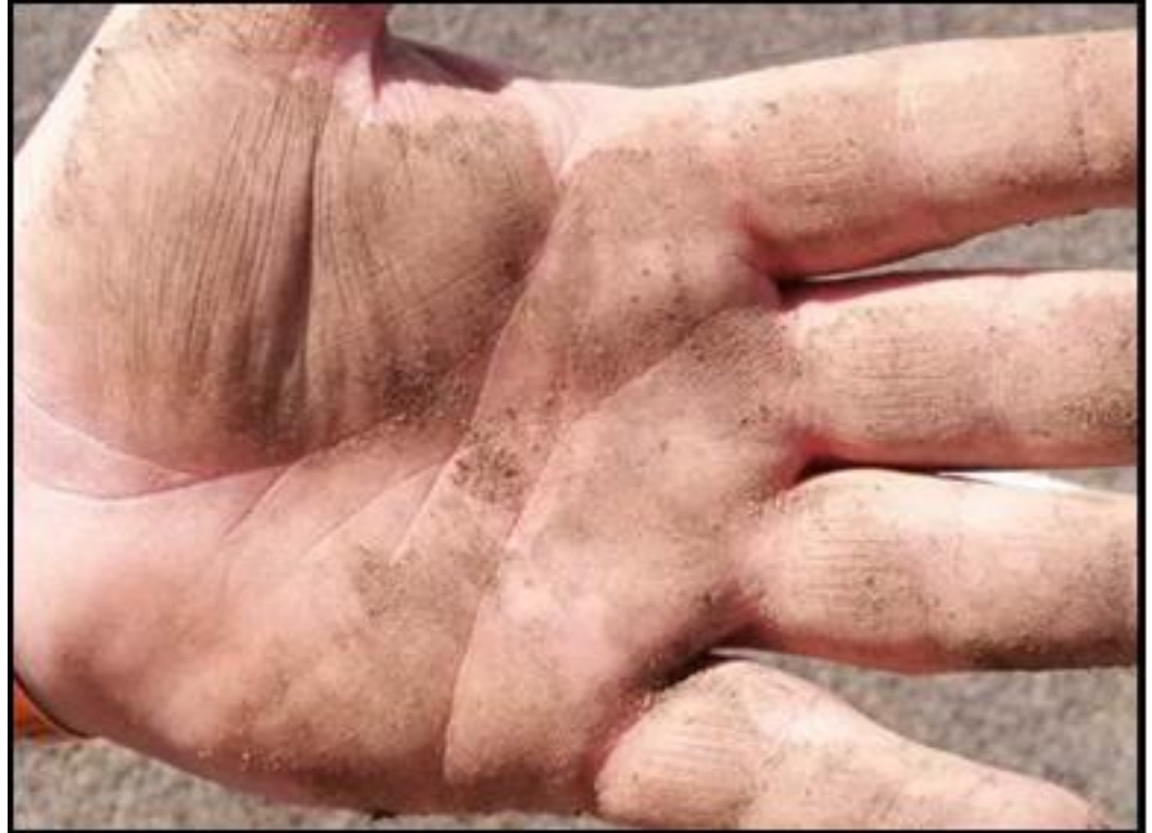
Figure 13: Demonstration of the effect of the organofunctional modification of the anionic bitumen emulsion used in the NME pothole kits that is designed to adhere to granular material, resulting in a minimum contamination when in contact with bare skin. No bitumen is sticking to the hand and the dirt can easily be washed using normal soap and water.
