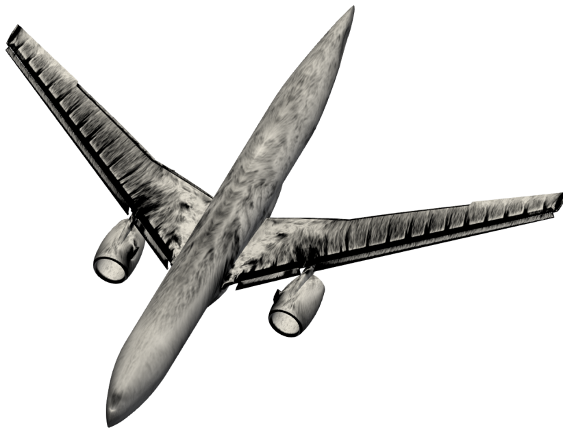
Figure 3. Prediction of the wall-shear stress in the High-Lift Common Research Model at an angle of attack of 21 degrees computed using wall-modeled large-eddy simulation with the Alya solver on a grid with 40 million control elements.
