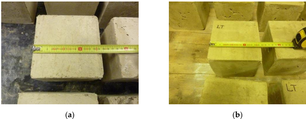
Figure 4. Dimensional check after drying: (a) TQ specimens; (b) LT specimens.
