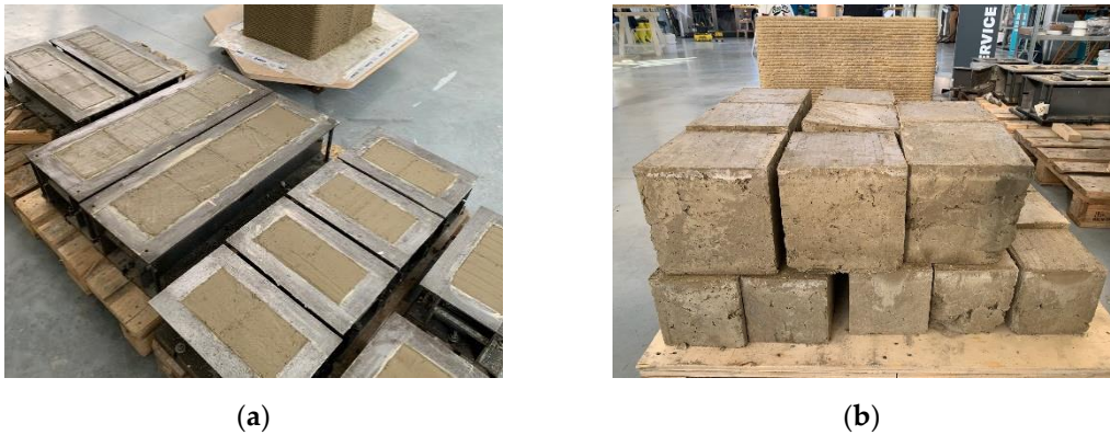
Figure 3. Preparation of the specimens: (a) The specimens after casting in the formworks; (b) Appearance of the specimens upon removal of the formworks (before the selection that led to the exclusion of some specimens).
