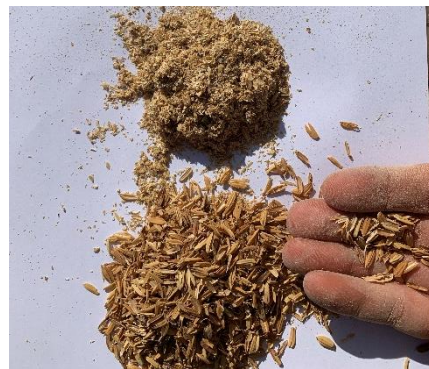
Figure 2. The two types of RH used in the experimental program, arranged with decreasing particle size from bottom to top: unaltered RH (maximum size variable from 6 to 8 mm) and shredded RH (maximum size: 2 mm).
