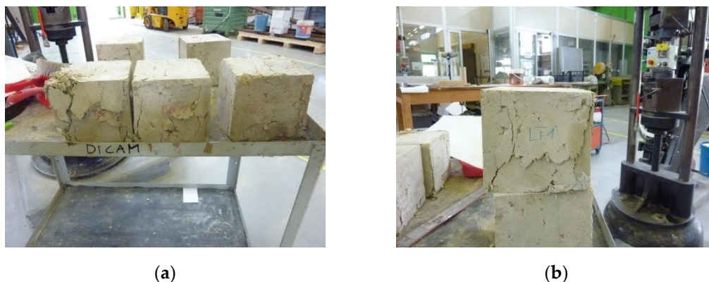
Figure 10. Appearance of the specimens after removal from the testing machine: (a) Three TQ specimens in the foreground; (b) Detail of an LT specimens.
