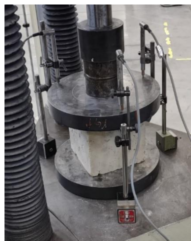
Figure 5. Placement of the three LVDTs on the bottom plate of the testing machine.
