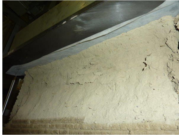
Figure 26. Appearance of the extruded layers along one of the sliding surfaces activated by crack propagation.
