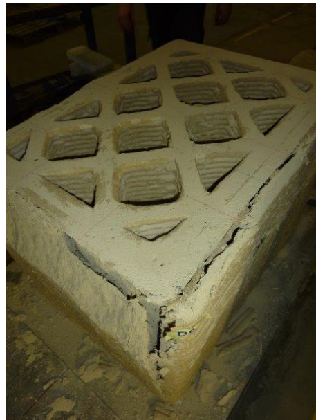
Figure 22. Appearance of the specimen after raising the head of the testing machine.
