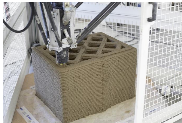
Figure 3. The 3D printing of the specimen object of this paper.
