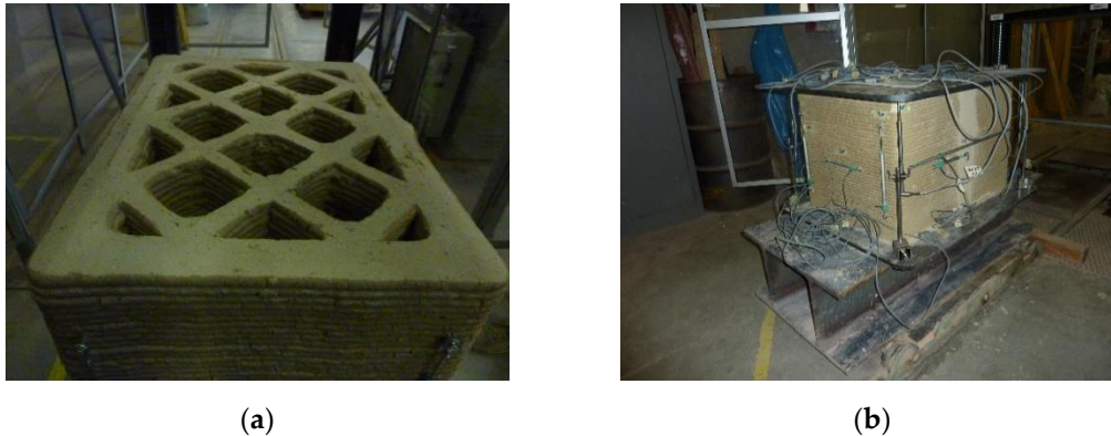
Figure 6. The specimen after hand sanding: (a) On the upper face; (b) On the long side face facing the operator.
