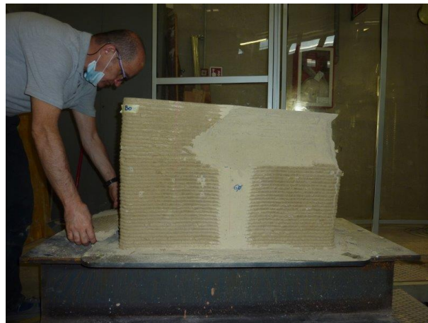
Figure 11. Front view of the specimen after the load test, with the upper face permanently inclined from left to right.
