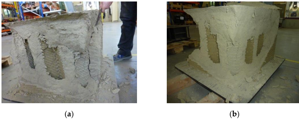
Figure 23. Side views of the specimen after the test: (a) Before and (b) after the removal of the material isolated (only in part) by the sliding surfaces.
