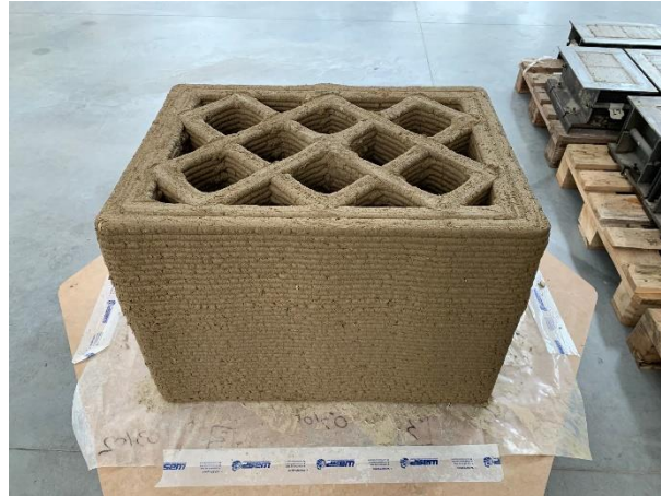
Figure 4. 3D printed specimen in the fresh state.
