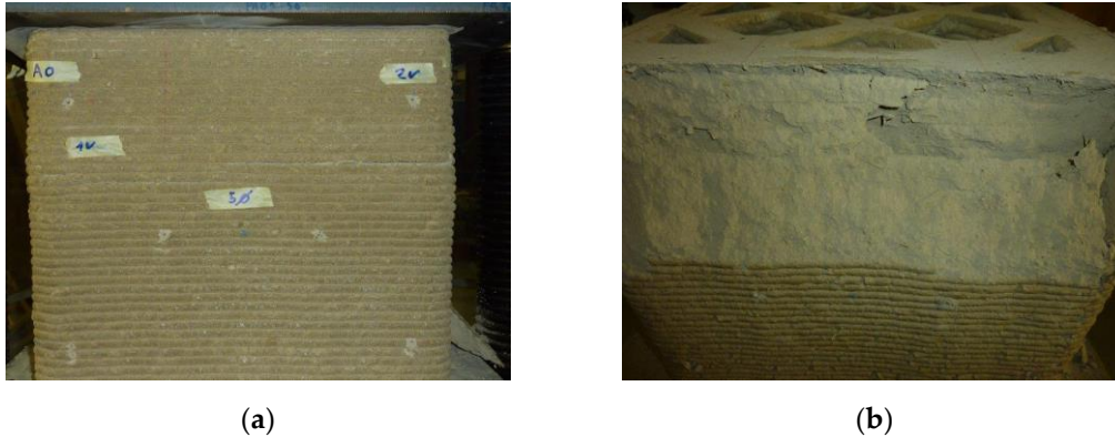
Figure 9. Failure mechanisms on the two short sides: (a) Side located to the left of the operator, extending between edge 1 (left) and edge 2 (right); (b) Side located to the right of the operator, extending between edge 3 (left) and edge 4 (right).
