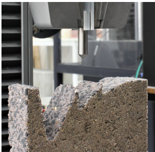
Figure 4. A photo of the Instron driving a tip against concrete
