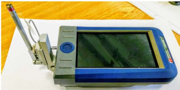
Figure 6 The Taylor Hobson Surtronic S-128 roughness tester used.
