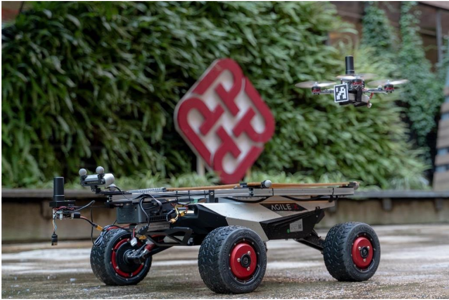
Figure 1. Prototype of the proactive guidance UGV and the UAV.
