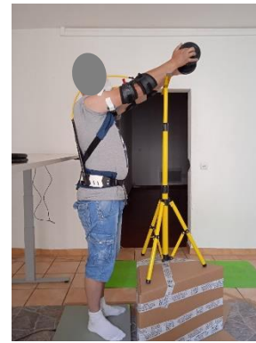
Figure 1: static task with arms at 105^\circ , 1 kg per hand
