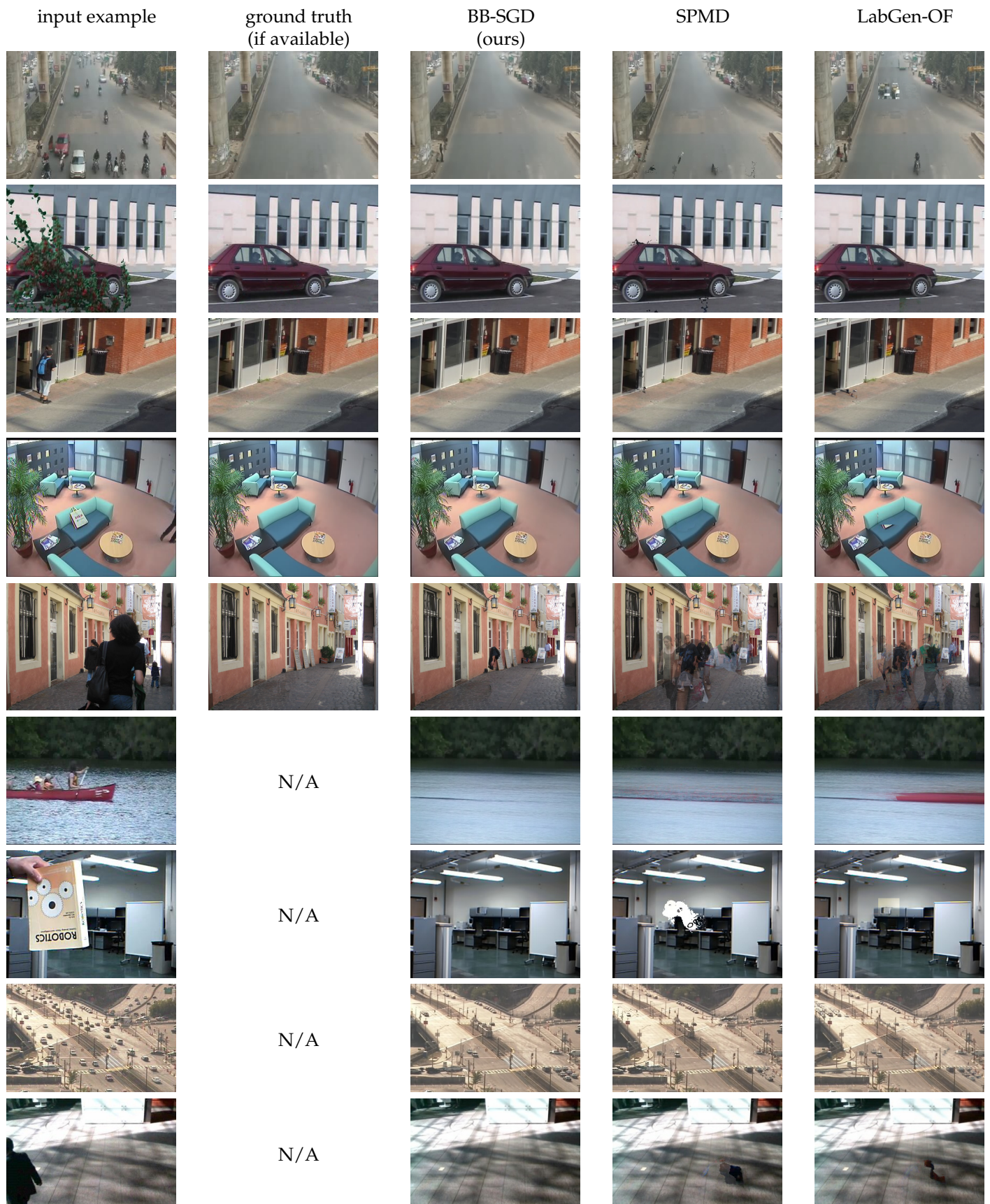
Figure 2. examples of background reconstruction using the proposed model and comparison with SPMD and LabGen-OF
