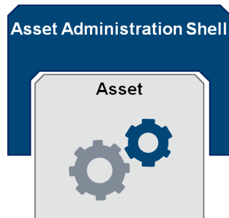
Figure 1. Representation of an I4.0 Component (I4.0C) composed of the asset and the Asset Administration Shell (AAS).
