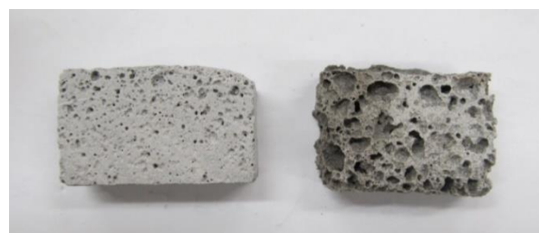
Figure 2. Foamed sodium (left) and potassium (right) geopolymer
