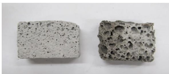
Figure 2. Foamed sodium (left) and potassium (right) geopolymer
