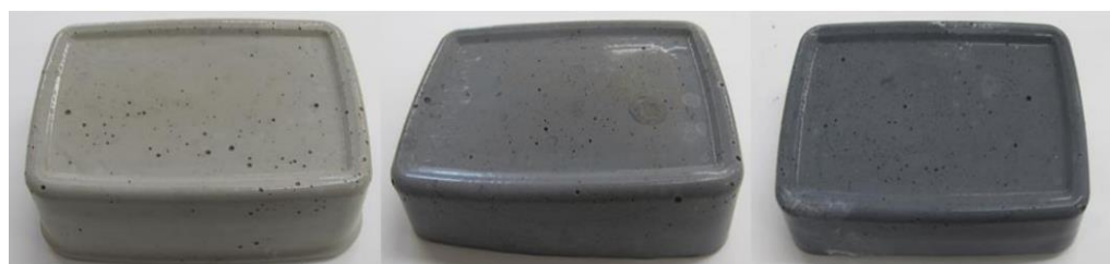
Figure 1. Geopolymers with 0 wt. %, 5 wt.% and 10 wt.% of high-carbon fly ash
