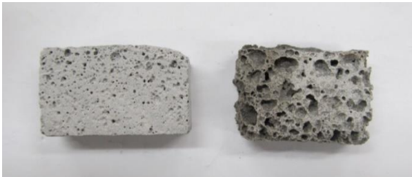
Figure 2. Foamed sodium (left) and potassium (right) geopolymer
