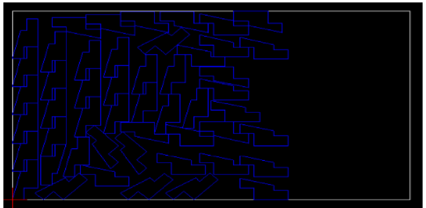
Figure 19. Final result when performing the nesting of case study 4 with a rotation step of 45^\circ .
