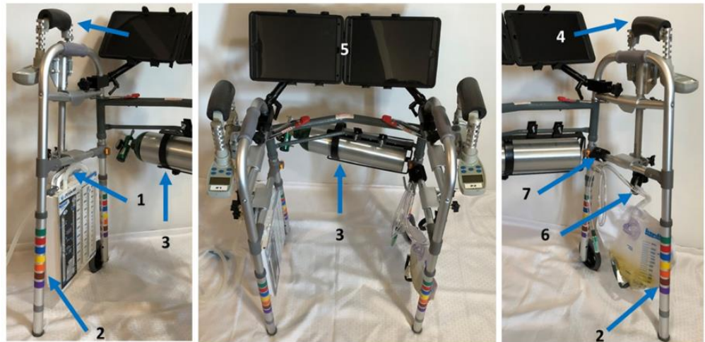
Figure 2. Clinical Force Measuring Walker v1.0 components: 1) Chest tube reservoir plate, 2) Color coded walker legs, 3) Oxygen tank mounting bracket, 4) Ergonomic soft handle grips, 5) Tablet adjustable mounting arms & waterproof cases, 6) Urinary collection bag swivel hook, 7) Foley Catheter S-hook.
